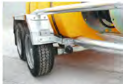
SIDE REFLECTOR AND TRAILER LIGHTING CONNECTION
